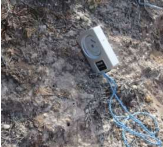
Figure 9: The use of a Silva clino-master Clinometer to measure the inclination of a burrow (Spiers, 2016h).
